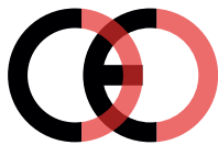
False CE Mark (too close)
