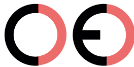
False CE Mark (too far)
